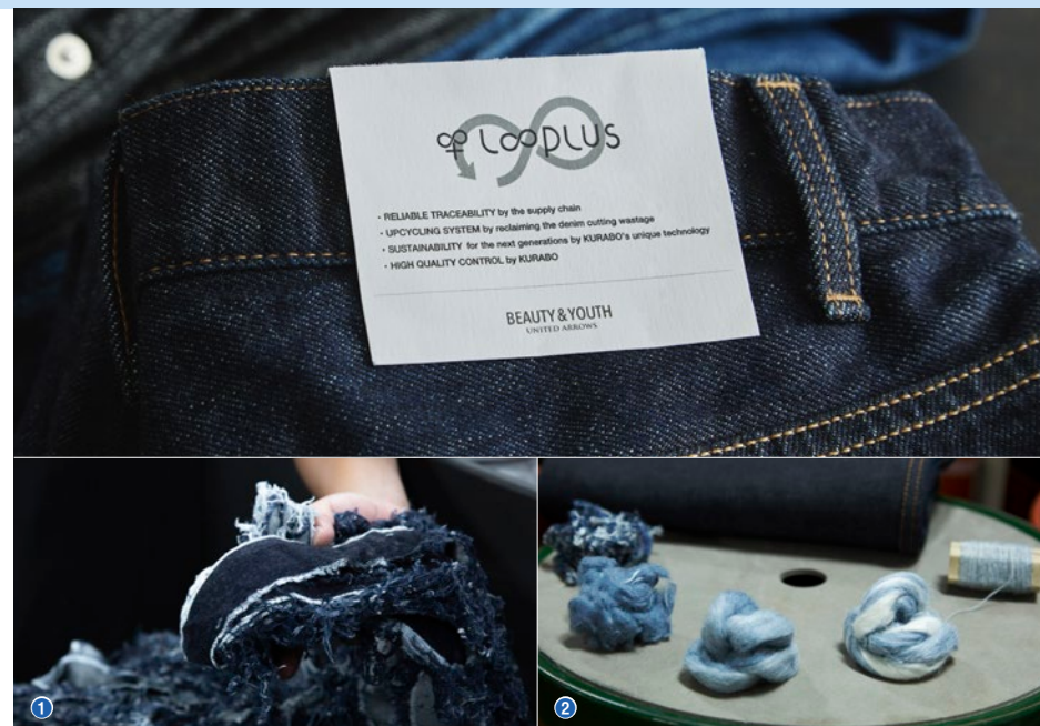
① Denim cutting waste used as raw material ② Process to form L∞PLUS yarn
